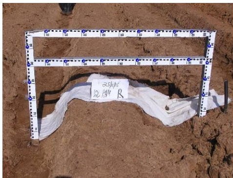
Fig. 4. Detected reference points – 24 points overall (marked by blue circles), all are inliers.
