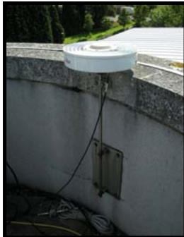
**Figure 3-1:** An AT503 Choke Ring Antenna Located at a Known Point on the Roof of the IESSG Building.
