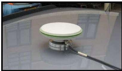
**Figure 3-3:** AT502 DF Antenna Installed on the Roof of a Car for the Kinematic Tests.
