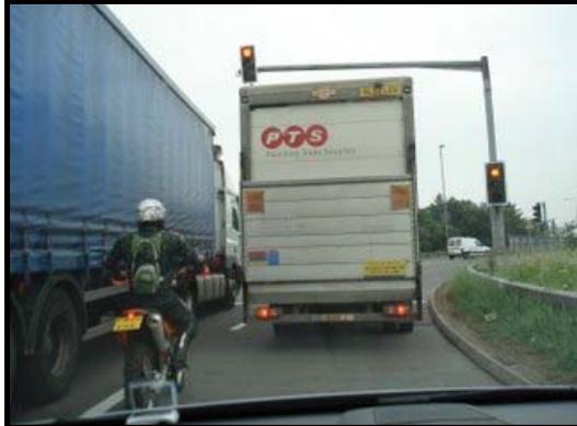
**Figure 4-10:** Lorries in the M1 Motorway Blocked GPS Signals and Caused Dynamic Multipath.
