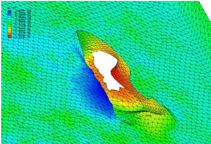
**Fig.3.** A 3D model of post-exploitation chambers on –100 to – 122-m level.
