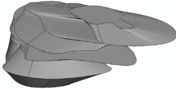
**Fig. 1.** Post-exploitation chambers measured with an echo-sonar
