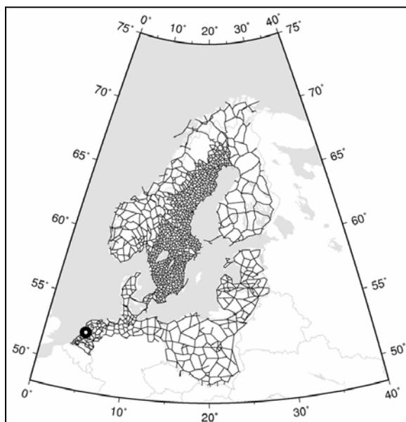
**Figure 4-1:** The Baltic Levelling Ring network. The zero point of it, NAP, is marked as a black ring on the map. (Mäkinen et al, 2005)
