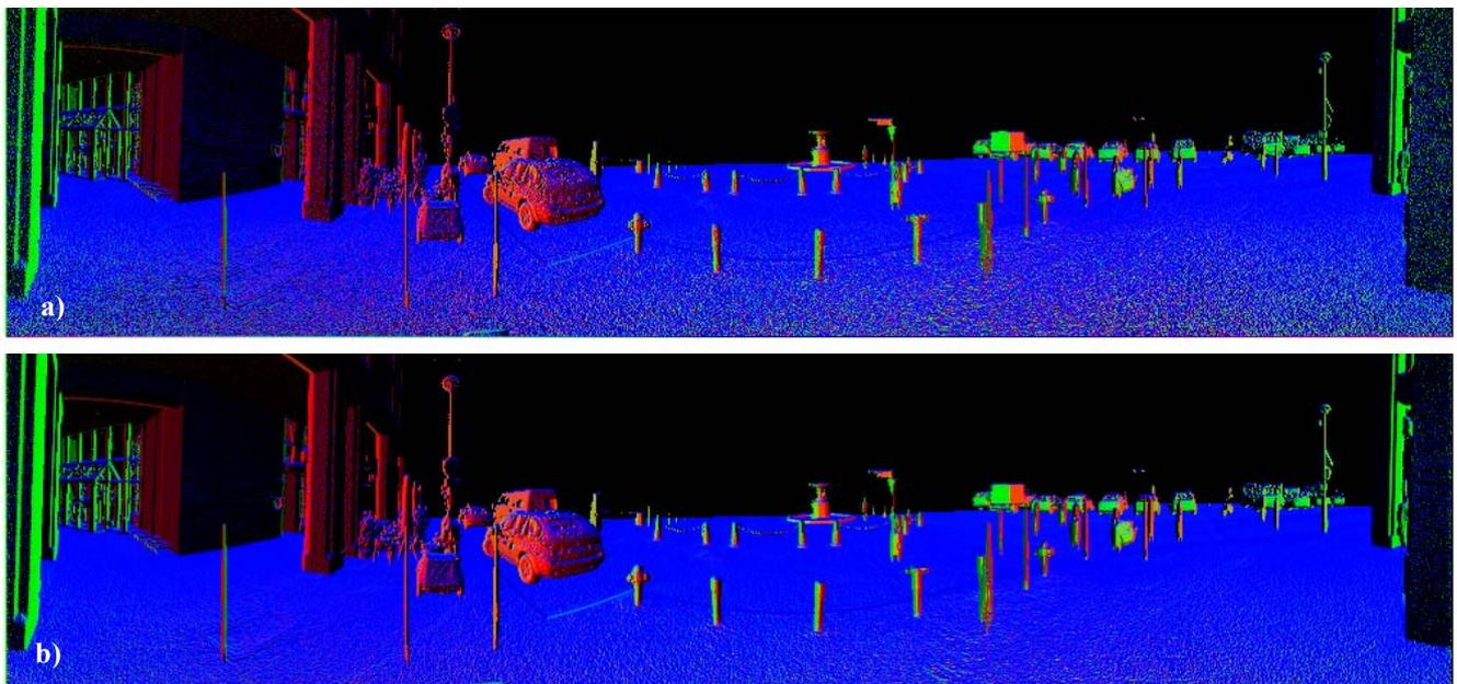
**Figure 8:** Normal vectors' direction, **a)** before and, **b)** after applying the adaptive smoothing procedure.
