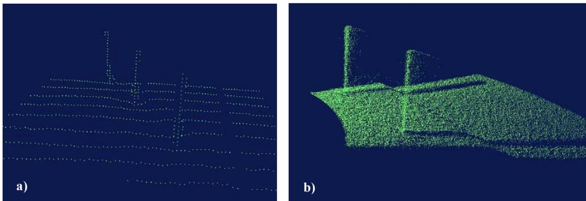
**Figure 1:** representation of similar objects located at different depths within the scan (25 and 2 m respectively).
