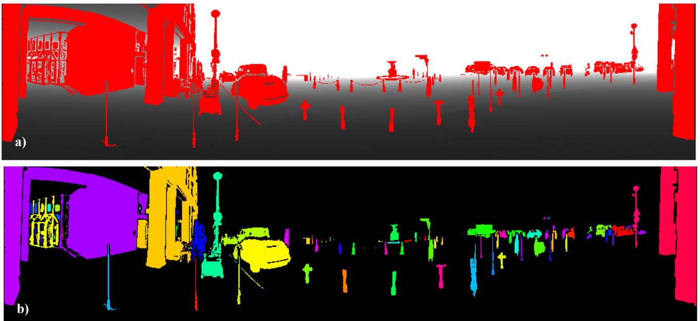
**Figure 10:** a) Object extraction results. b) Objects separation according to changes in depth.
