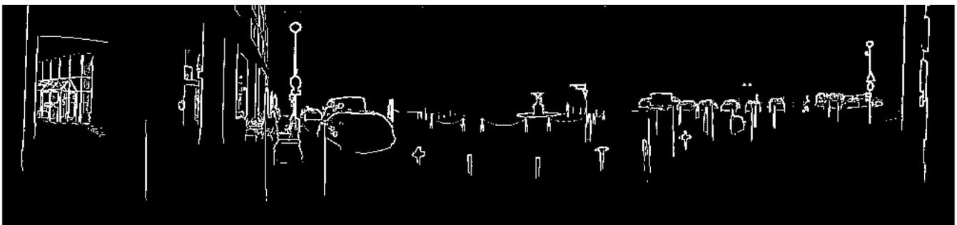
**Figure 3:** Edge detection using the application of the LoG operator on the range panorama.
