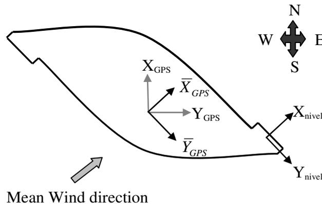
Figure 6. Plan view of the building & GPS and Nivel axes orientation with respect to building
