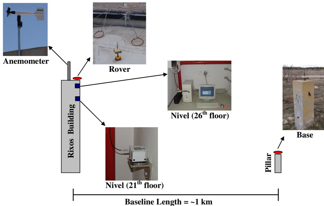
Figure 2. Schematic overview of GPS, inclinometer and anemometer deployment in the building.
