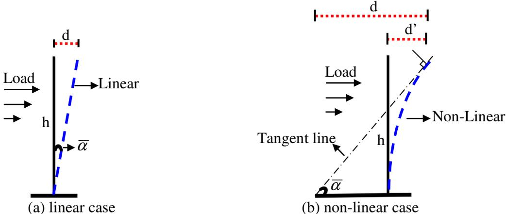
Figure 8. Illustration of converting inclination into displacement
