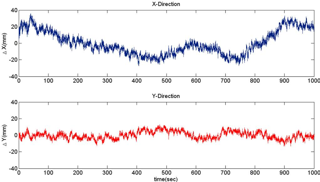
Figure 7. Kinematic GPS displacement time series
