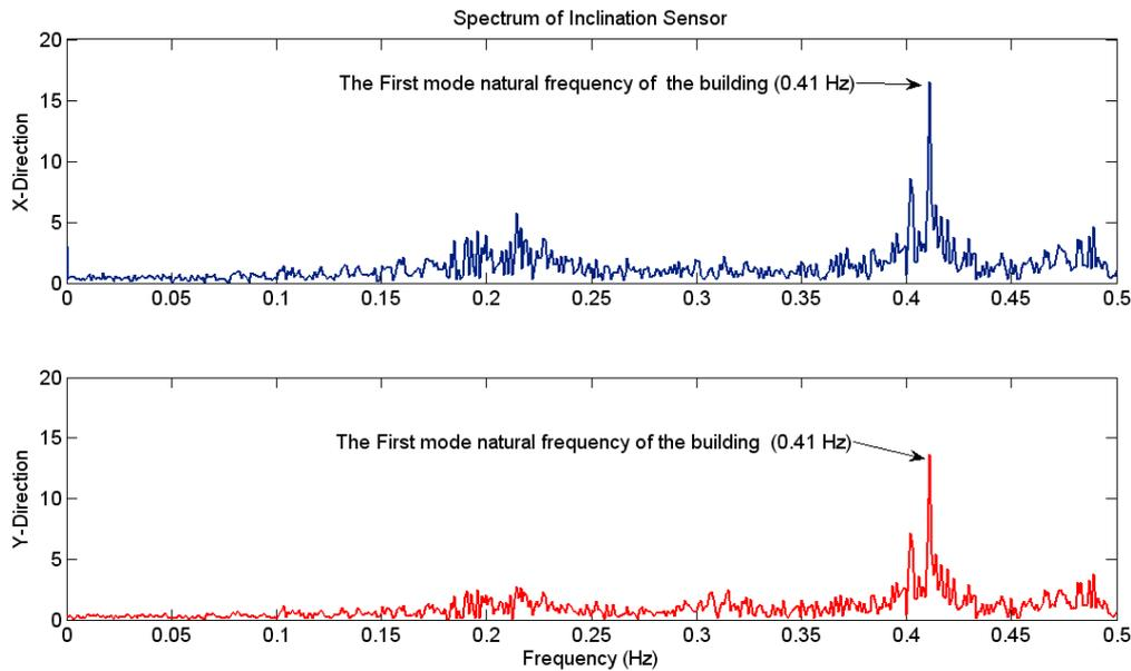
Figure 13. FFT Spectrum of Inclinometer Derived displacement time series
