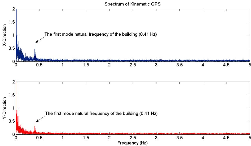
Figure 11. FFT Spectrums of Kinematic GPS Time Series for X & Y directions
