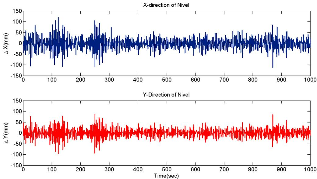
Figure 10. Inclinometer-derived displacements time series
