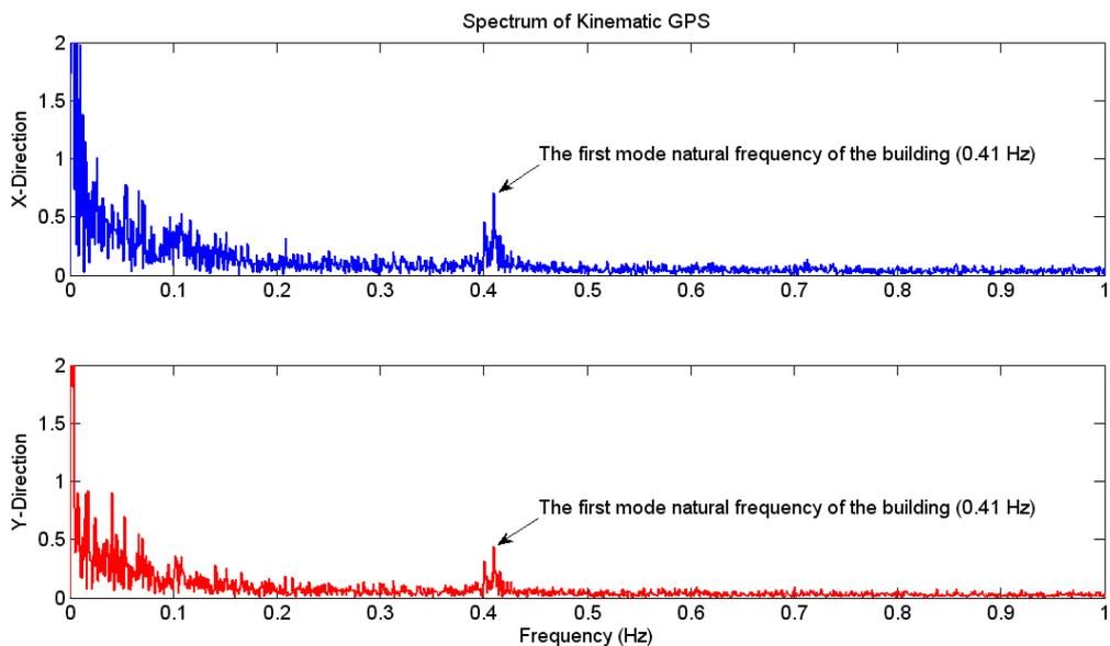
Figure 12. Zoom in of the FFT Spectrums of Kinematic GPS Time Series
