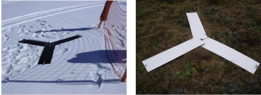
Figure 2: (a) (left) Black target for *snow* photography – *Campaign 2*, August 2007 and (b) (right) White target for *no-snow* photography – *Campaign 4*, November 2007.
