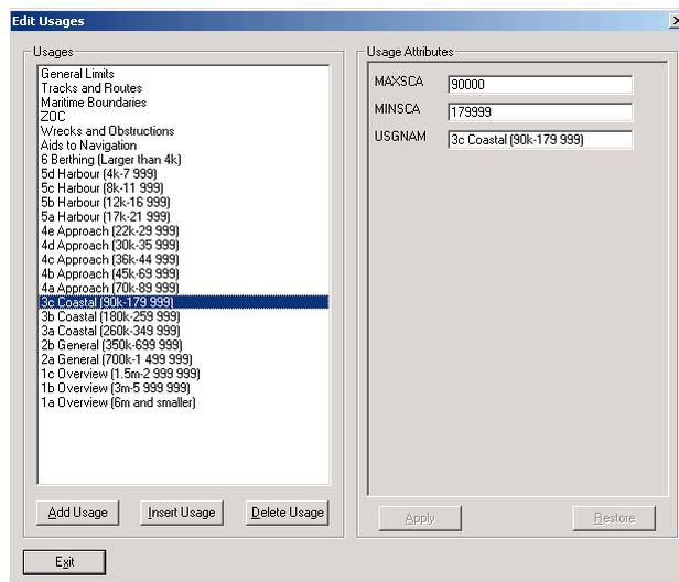
A number of 'scale-less' usages were also created, including: Aids to Navigation, Wrecks and Obstructions. The 'best scale' versions of point objects for these features are stored on these usages. While not truly scale-less, the HPD system allows representations at different scales to be created from these features. Assigning representations from these usages makes update
