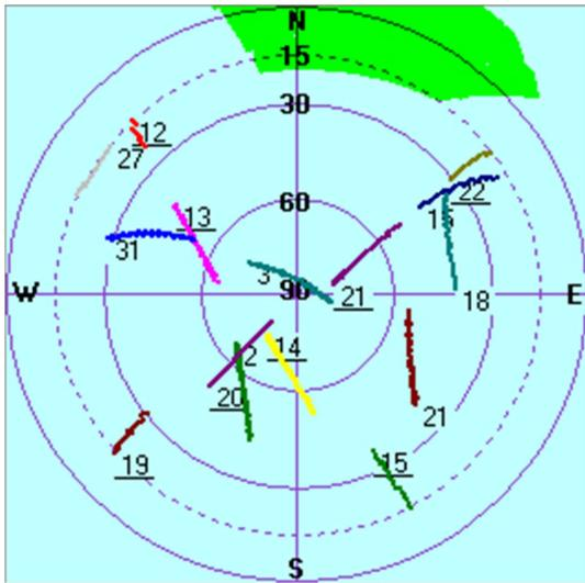
Fig.1. Sky plot of Galileo (underlined) and GPS satellites; the green area represents the reflector .
