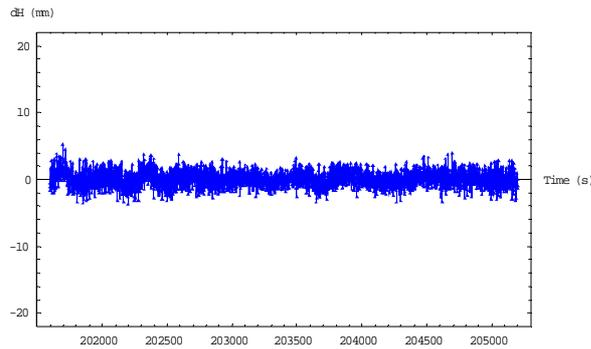
Fig.6. Positioning error in northing (top), easting (middle), and vertical (bottom) of single-epoch solution using Galileo + GPS three-frequency data.
