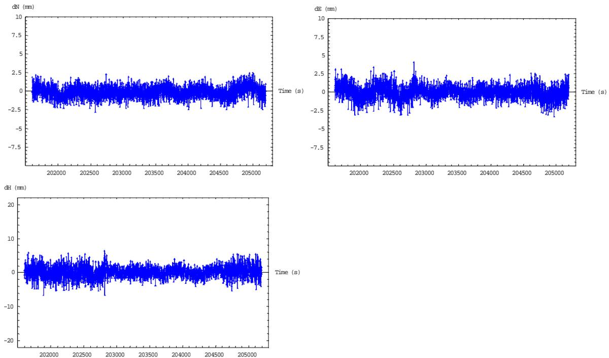
Fig.5. Positioning error in northing (top left), easting (top right), and vertical (bottom left) of single-epoch solution using Galileo three-frequency data.
