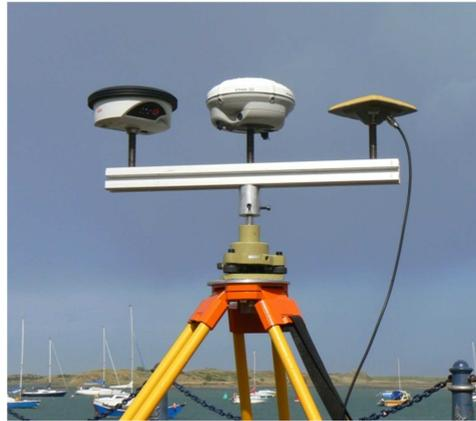
**Fig. 5:** Bracket allowing simultaneous observation with three receivers.
