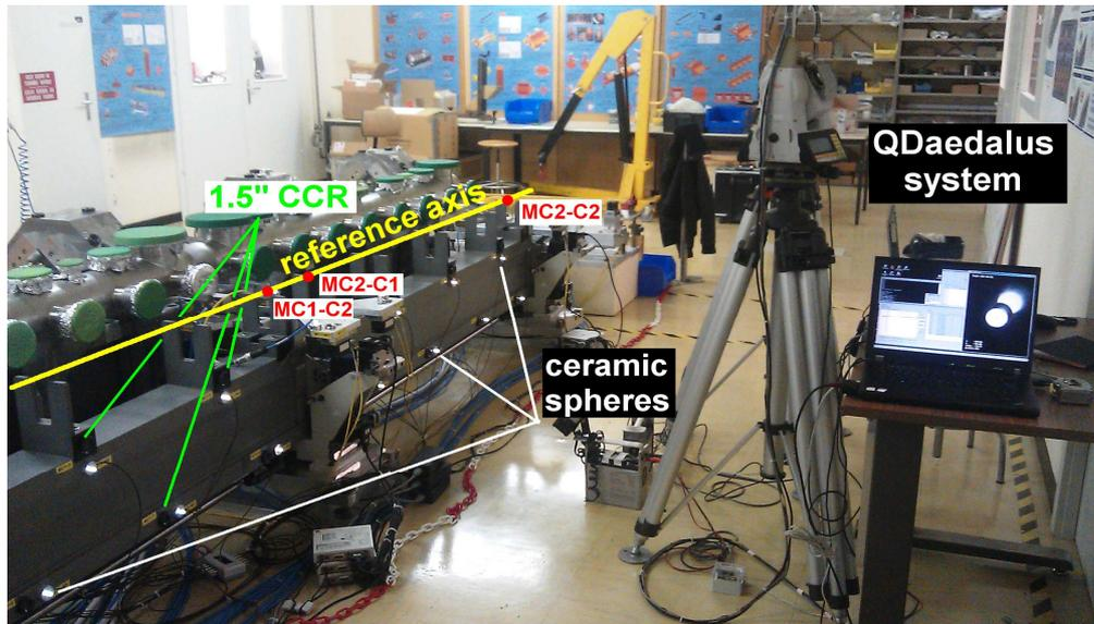
Figure 5. Photography of a part of the modules and the fiducials and one QDaedalus system installed at CERN in Geneva.
