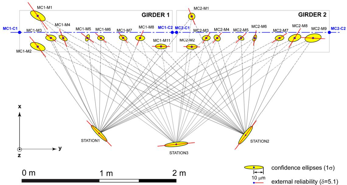
Figure 6. Microtriangulation Network measured with QDaedalus with the confidence ellipses and the vector of external reliability. The datum was fixed by minimizing the trace of the coordinates of all points on the modules.
