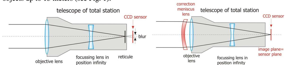
Figure 1. (Left) Removing the eyepiece and mounting a CCD sensor instead evokes optical blur at distances beyond 13 meters. (Right) Mounting a meniscus lens in front of the telescope objective moves the focal plane about 4 mm to the CCD sensor plane thus producing perfectly focused images
