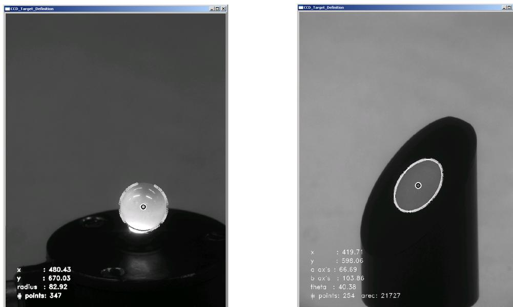
Figure 4. (Left) Example of an illuminated ceramic sphere measured with the circle matching algorithm. (Right) Example of a
