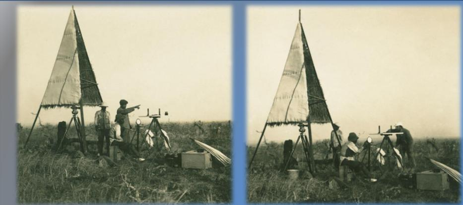
The alidade's observations were completed by telemeters (distances) and barometers (heights) measurements. The toponymy was collected in the villages.
