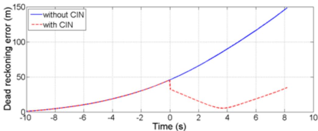
Figure 10: The performance of dead reckoning with and without CIN.
