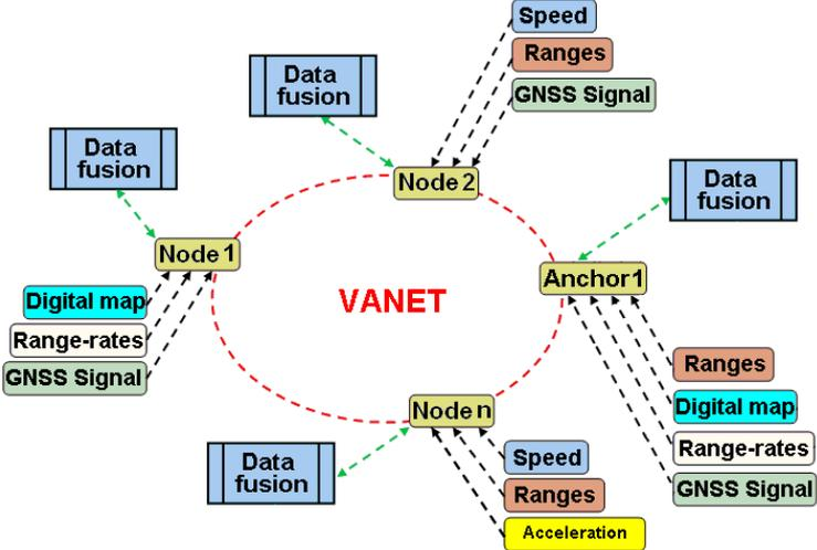
Figure 2: CP positioning architecture.
