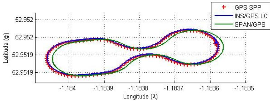
Figure 6: Train trajectory for MEMS INS testing
