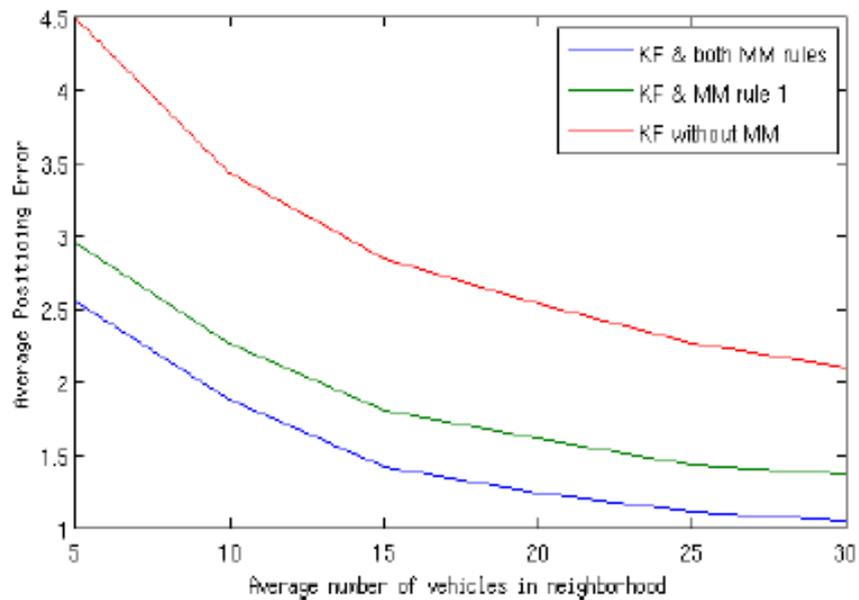
Figure 9: Simulation result shows that KF with both MM rules have better performance than KF with second MM rule only and KF without MM.
