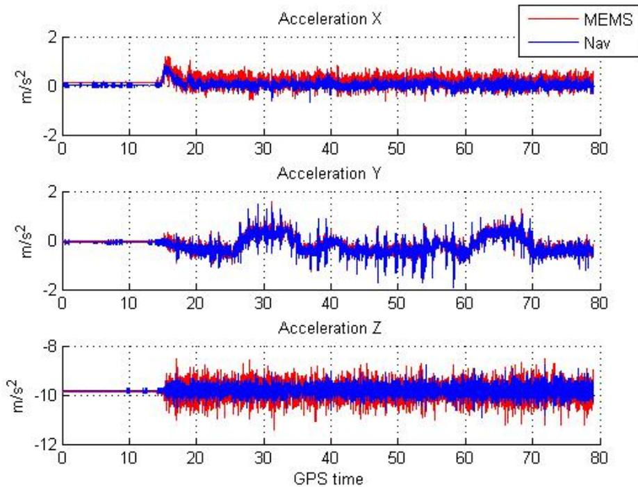
Figure 4: MEMS INS performance tests - accelerations.
