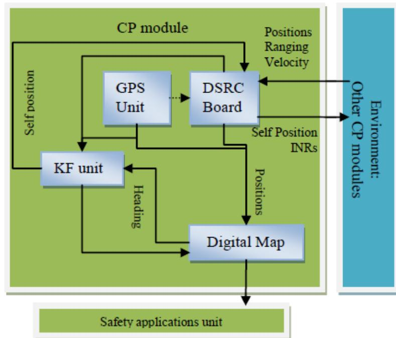
Figure 8: A CP module, consisting of positioning device (GPS unit), communication and ranging device (DSRC), computational processor (KF processing unit) and digital map.
