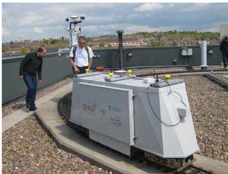
Figure 3: Train trajectory for MEMS INS testing
