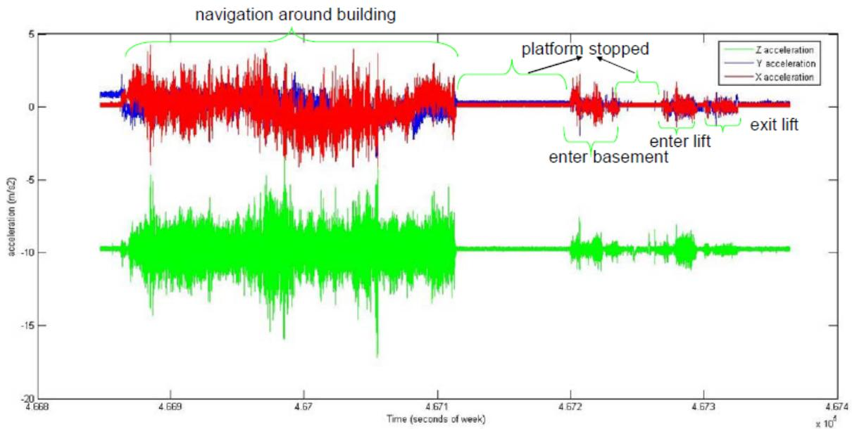
Figure 7: Qualitative information extracted from noisy MEMS data
