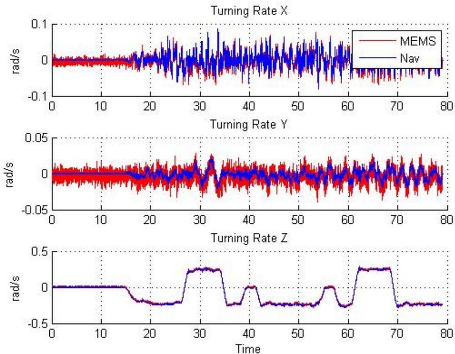
Figure 5: MEMS INS performance tests - turning rates.
