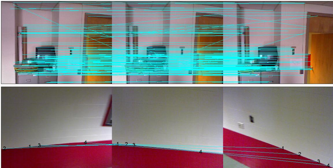
Figure 4: SIFT feature extraction and matching examples; top row shows normal situation, while the point distribution and image overlap are weak in the bottom row.
