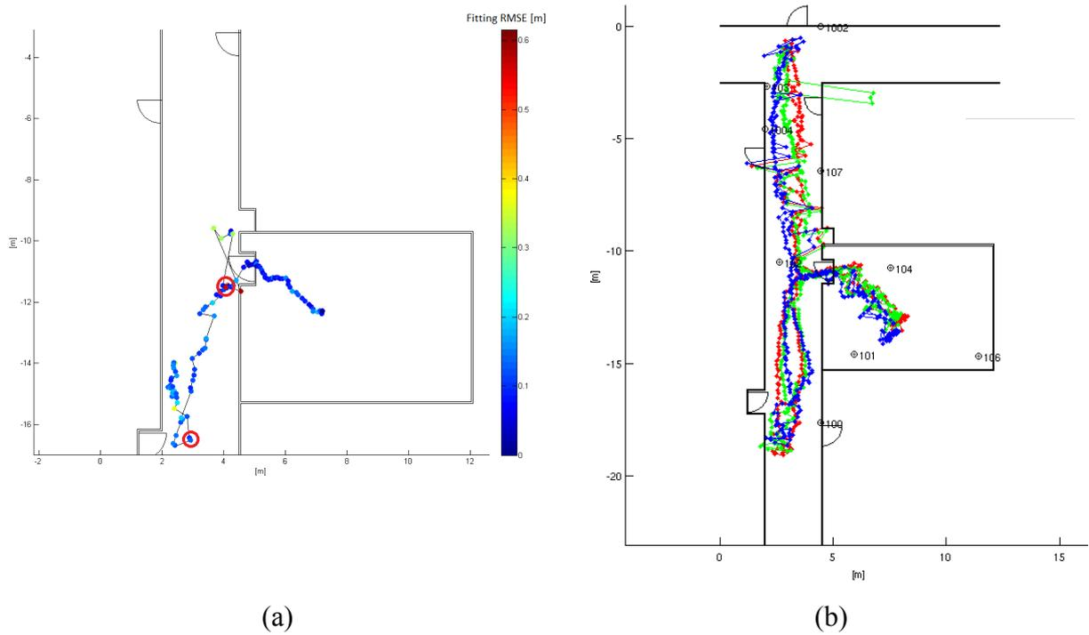
Figure 6: Trajectory evaluation; (a) combined 2D and 3D image based trajectory reconstruction, and (b) UWB reference solutions.
