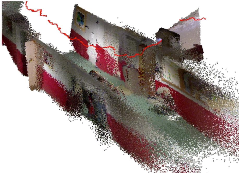
Figure 7: Stitched point cloud (ceiling removed) and reconstructed trajectory (red).
