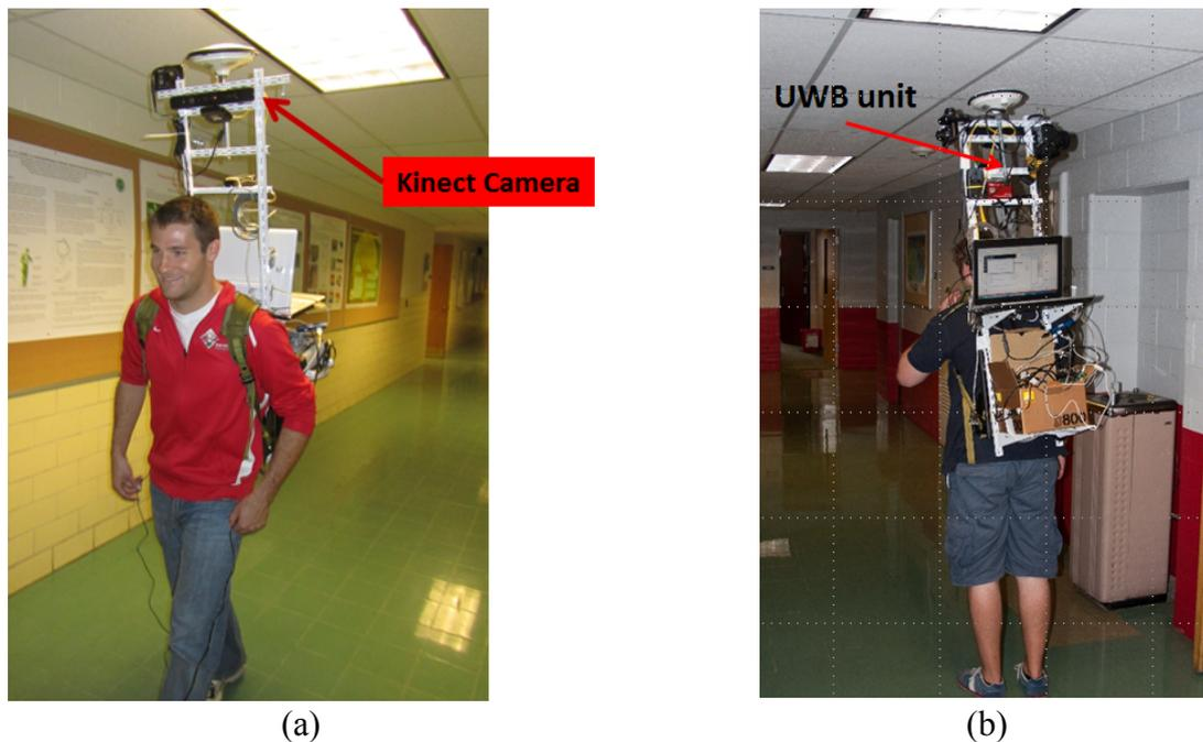
Figure 3: OSU backpack personal navigator prototype; (a) Kinect™ and (b) UWB sensor.
