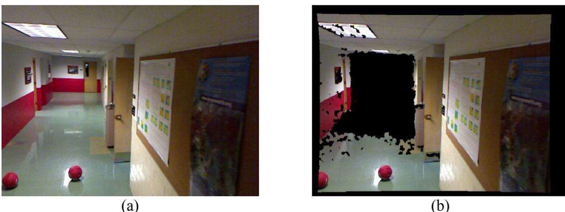
Figure 2: Kinect™ images; (a) RGB and (b) colored 3D depth image.
