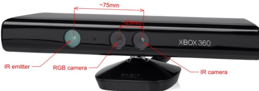
Figure 1: Kinect™ sensor.
