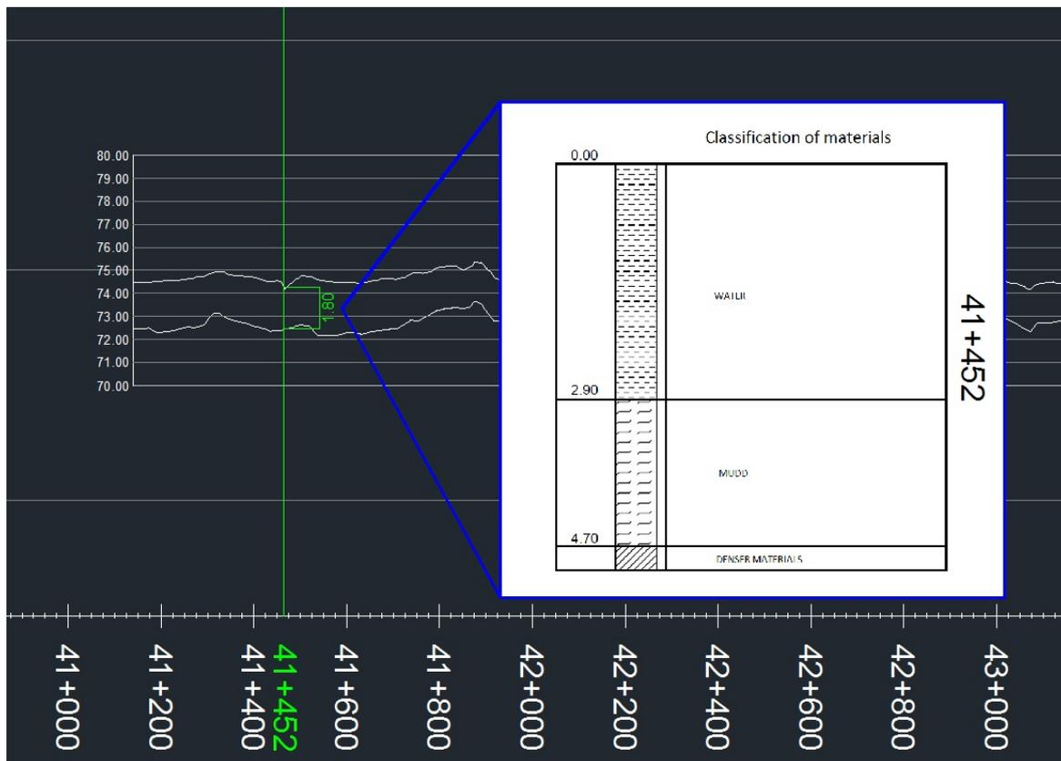
**Figure 5.** Correlation between the mud thickness determined by sub-bottom profiler and by geotechnical core sampling
