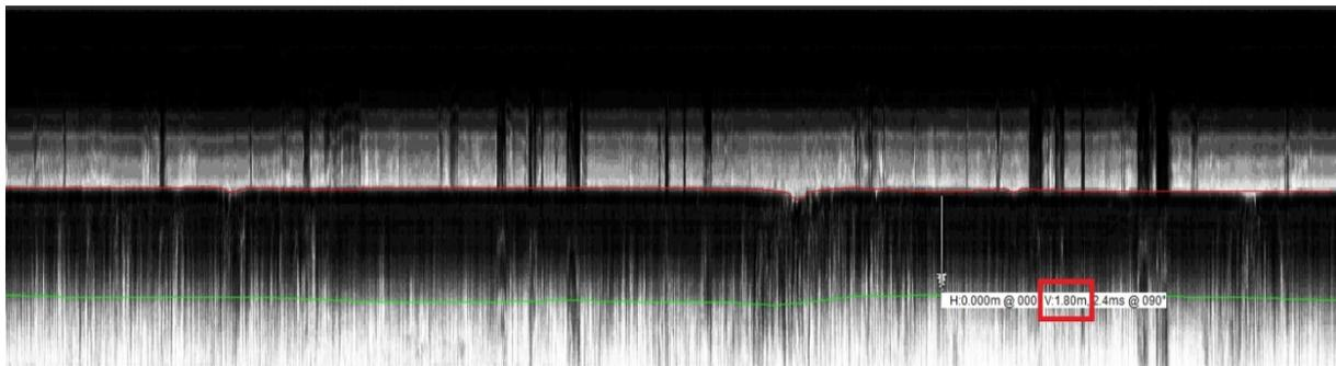
Figure 4. sub-bottom measurements being vectorized and showing the sediment thickness of 1.8 m.
