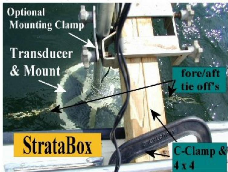
Figure 3. StrataBox overboard installation
