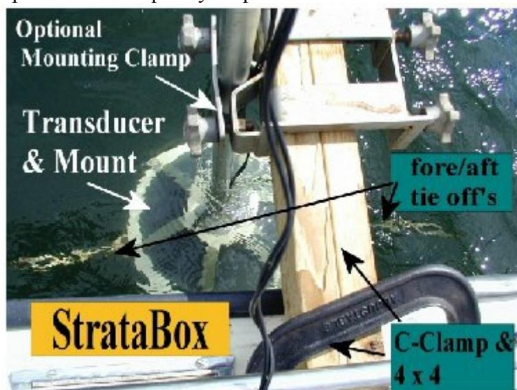
Figure 3. StrataBox overboard installation
