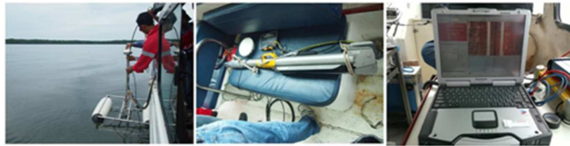
Side Scan Sonar survey - system onboard
