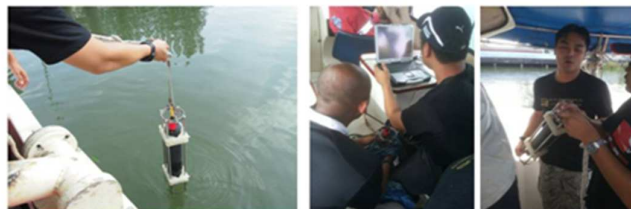
Sound velocity measurement using SVP
