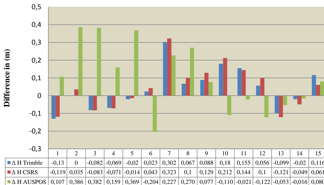
Figure 111: Height accuracy obtained via the three PPP online services using two-hour data
