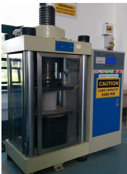
Fig. 6a: Compressive Strength Testing
