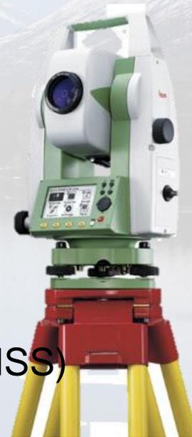
We set up the TST in different geo-referenced points (with GNSS) around the stockpile
