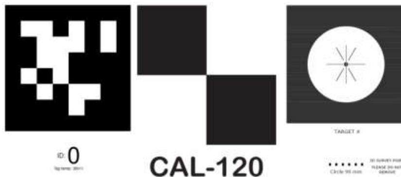
*Figure 3: particular of the target used (April tags, survey tags)*
