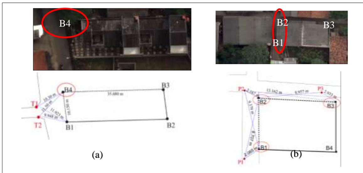
Figure. 3. (a) Determination of land parcel boundary B4 with metode of "pemotongan kemuka" (b) Determination of land parcel boundary B1, B2, and B3 with combination method of GNSS and Terrestriis
