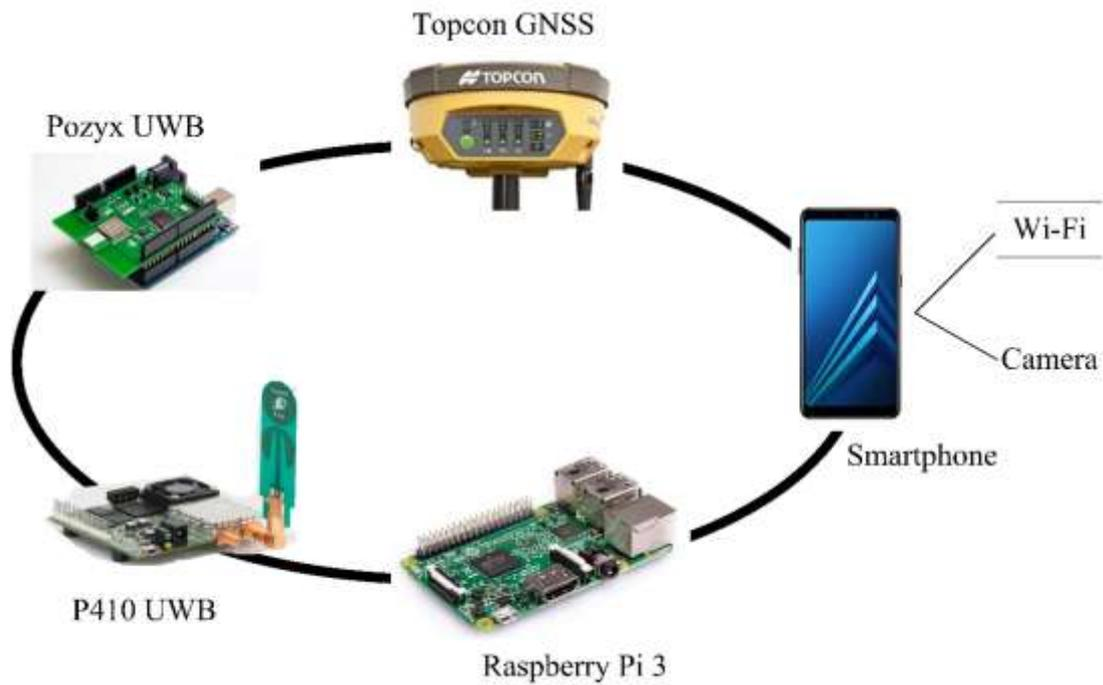
Figure 1: Overview of the sensors integrated on one of the pedestrian helmets in the developed system.
