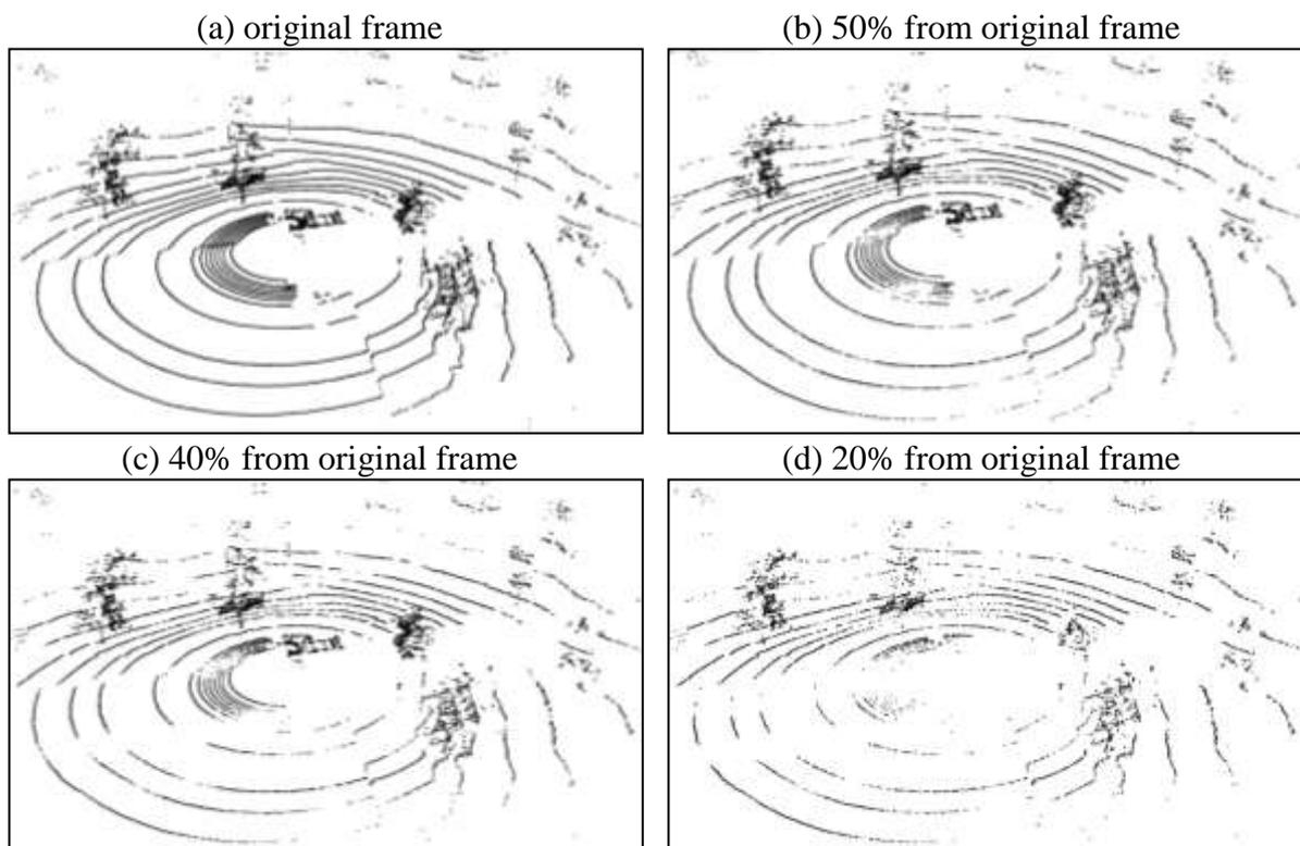
Figure 11: MLS data (a) original frame, (b) 50% of points after reduction, (c) 40% of points after reduction, (d) 20% of points after reduction.
