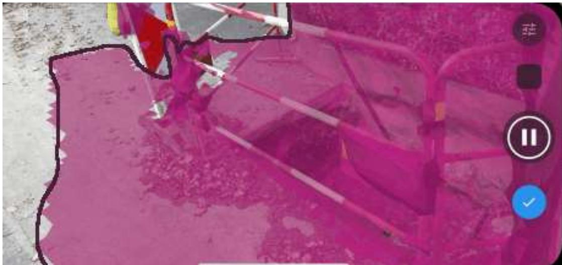
Figure 3. Pix4D catch during the acquisition of images. The purple area, enclosed in the black line, indicates to the user which portion of the site was already correctly acquired.
