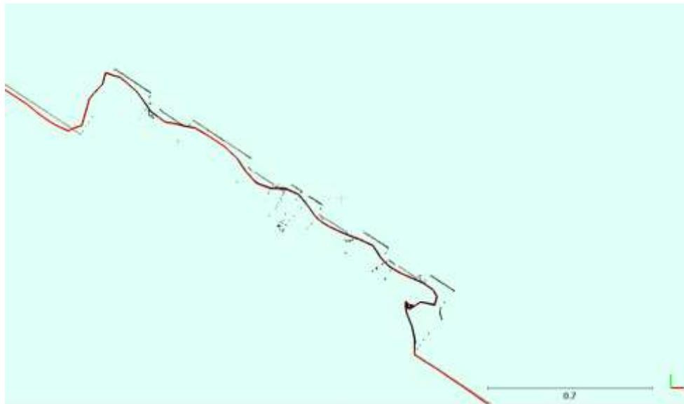
Figure 5. Focus of extracted horizontal sections. Red line: Canvas mesh; grey line: Faro point cloud
