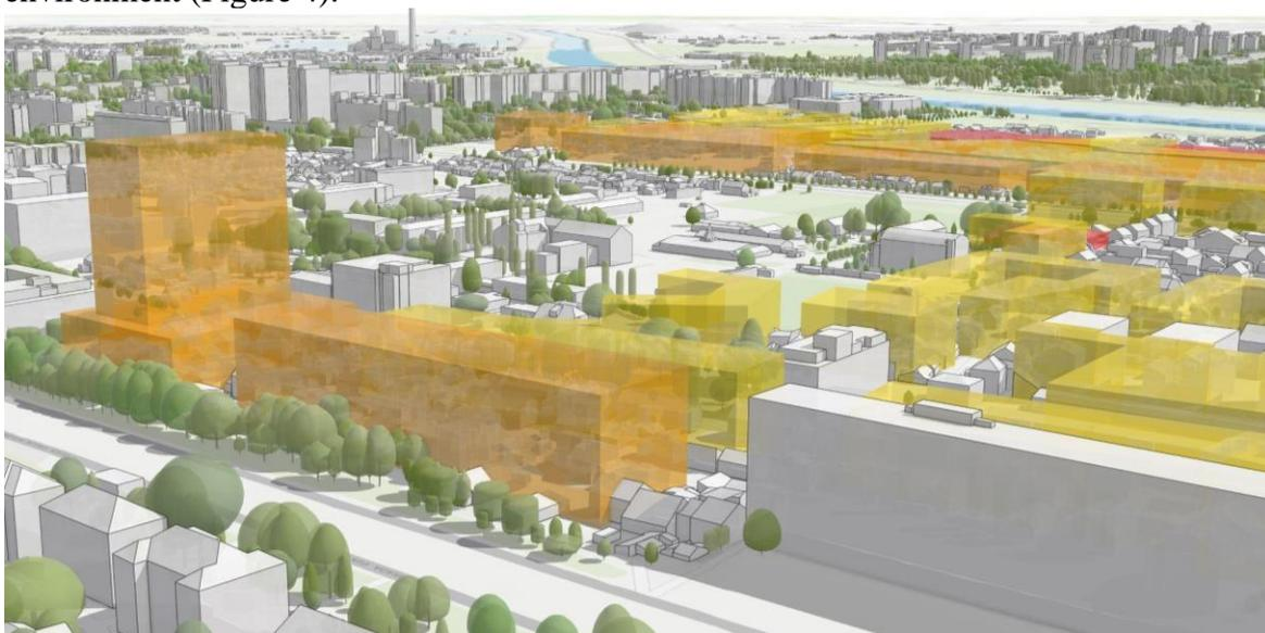
Figure 4. 3D building lines and volumes interpreted from detailed urban plan (Trnje, Zagreb)
