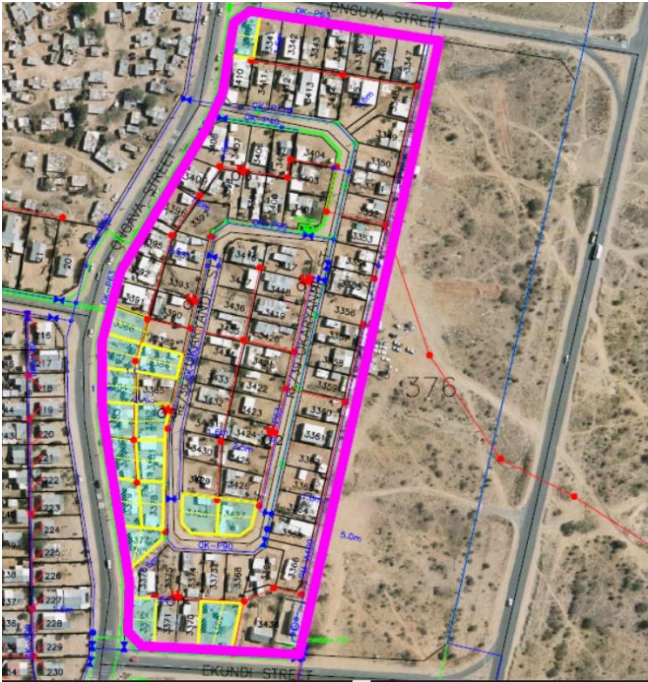
Figure 2: Layout plan prepared by the City of Windhoek for the formalisation of Tweetheni, here plots are demarcated, provision of bulk infrastructure is made and streets are clearly layout.
