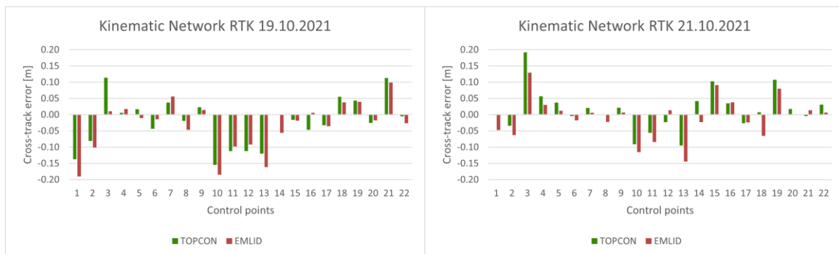
Figure 3. Cross-track errors computed in each control point for the network RTK solutions. Results for day 19.10.2021 left and day 21.10.2021 right.
