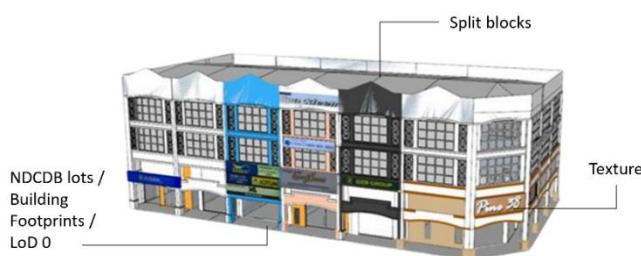
Figure 4: A 3D Model of a Shop House Block Segmented According to NDCDB Lots
