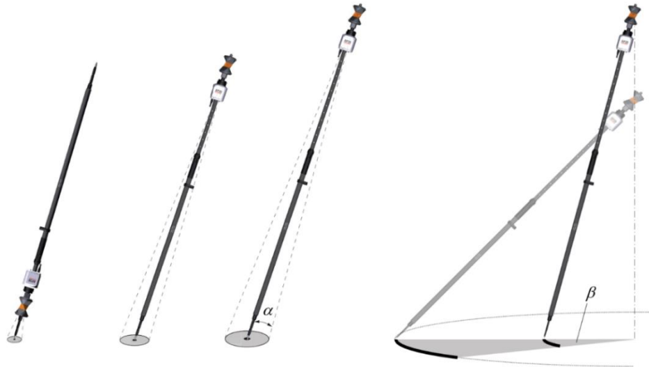
Figure 3 The smaller the target height, the smaller the projected footprint of a certain tilt error \alpha (see left). The smaller the tilt, the smaller the impact of a certain tilt direction error \beta (see right).
