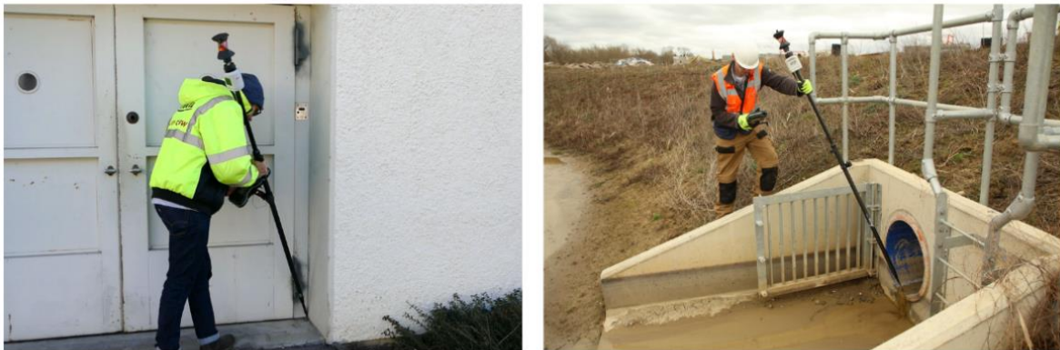
Figure 1 Examples of points which previously were impossible to measure with an upright levelled pole
