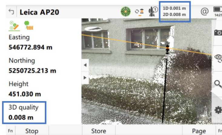
Figure 6 Real-time representation of the estimated overall coordinate quality of the pole tip (incl. target position and attitude quality) within Leica Captivate field software
