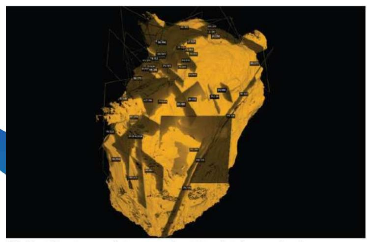
3HP's Olympic Dam mine stope analysis process involves picking geological structures from Hovermap scans. High-resolution final stope scans are imported into the mine's co-ordinate system before the geotechnical team picks the structures that control the final stope shape. (Source: BHP, Evan Jones, Emesent webinar.)
