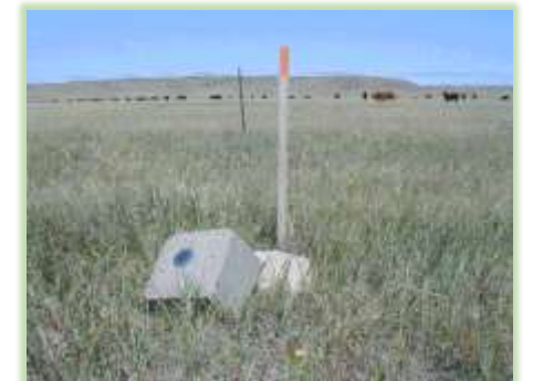
Destroyed Geodetic Control No Coordinates/Elevation!
