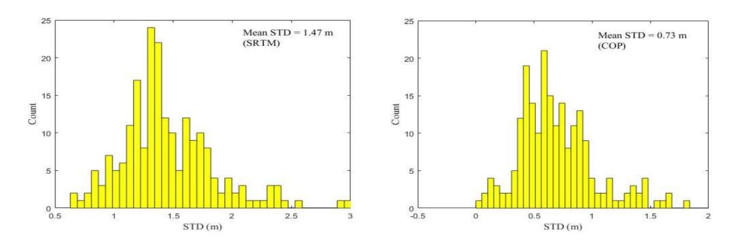
The relative vertical accuracy (one sigma) of SRTM is 1.47 m vs. COP is 0.73 m
