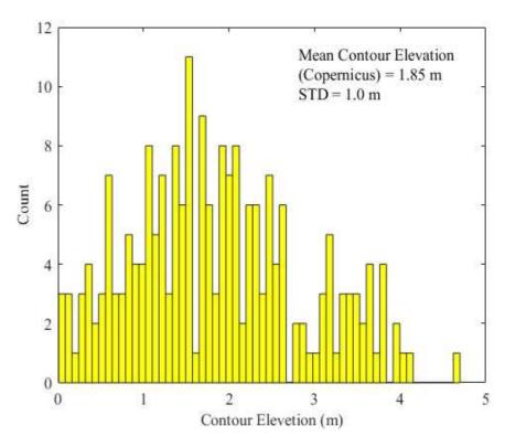
The average elevation of the SRTM-derived lines elevation is 2.63 m. while for the COP, it is 1.85 m. A vertical shift between SRTM and COP of 0.78 m is present.
