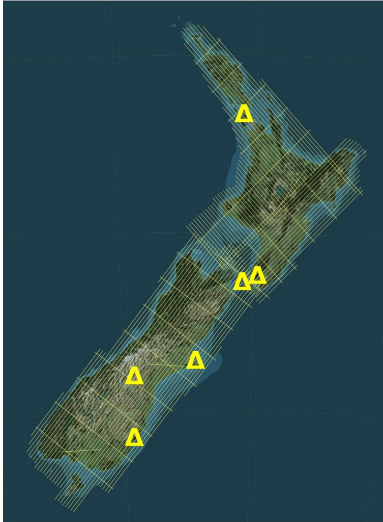
Diagram 4: The six absolute gravity sites shown as triangles, and flight lines from the 2014-2015 airborne gravity survey campaign that contributed to NZVD2016.
