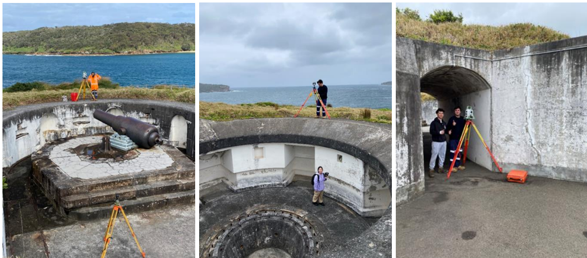
Figure 4 – a) Chasing the mms as part of the control survey; b) Control survey (top) and mobile laser scanning (below) showcasing the 3D nature of the survey; c) Control traverse around the tunnels for georeferencing targets.
