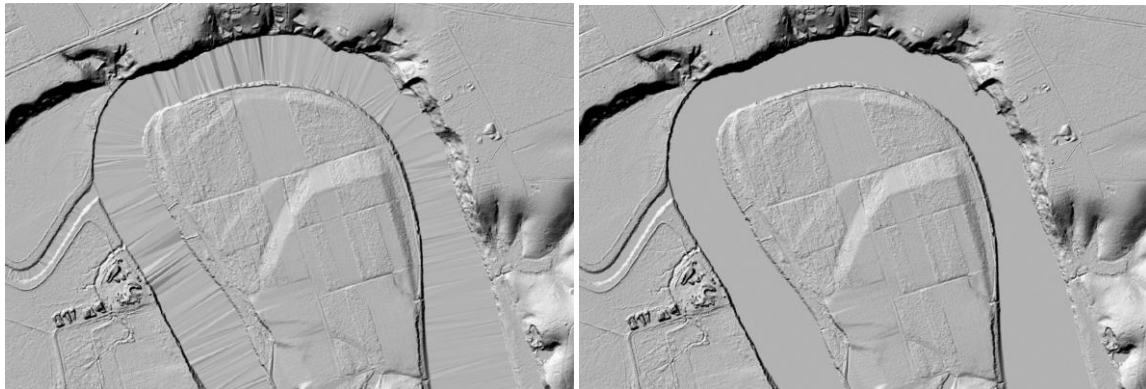
Figure 18: An example of non-hydro-flattened (left) and hydro-flattened (right) DTM.
