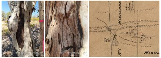
Figure 9 Photos of the Original Reference tree, HP14, found to reference station 235b on plan B144102 (extract of plan shown)
