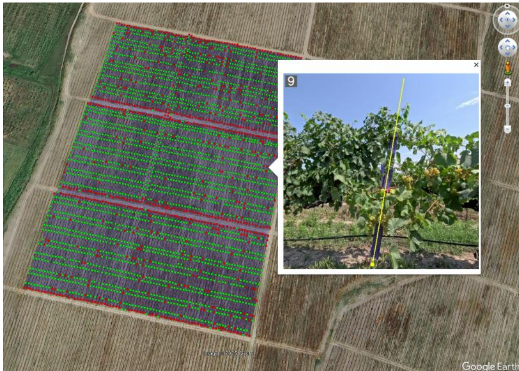
Figure 7: Example of pillars map with the ability to analyze pillars with a significant slope (problematic pillars are marked as red points)
