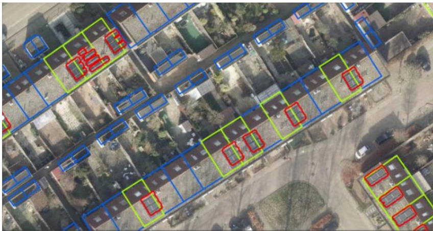
Figure 2: The detection of solar panels (red) on buildings. Based on these detections, buildings are classified as either possessing solar panels (green) or lacking them (blue).
