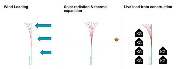
Figure 1 Environmental forces and live load impacting tall buildings
