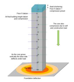
Figure 2 The effect of the load on tall buildings
