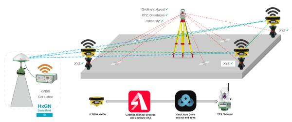
Figure 4 Core components of the Leica Geosystems' CWCS solution
