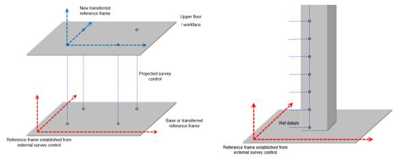
Figure 3 Transfer of the building's reference frame
