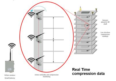
Figure 5 WiSenMeshWAN® solution for real-time compression readings
