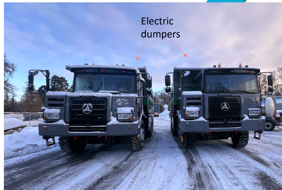
SANY - SKT90E Electric Off-Highway Mining Truck Load Weight 37 T
