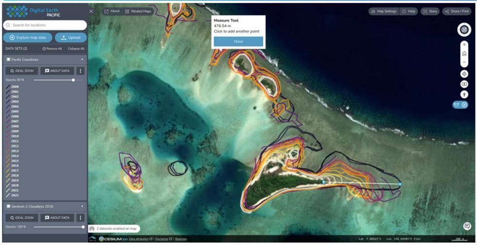
Landsat annual mosaics were created by calculating the median image values among times of near-average (0-m) sea level using a tidal model. A water discrimination technique was applied which allowed delineation of exact coastlines at the subpixel level.
