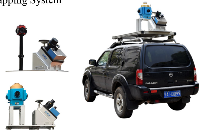
HiScan-Z High-Precision 3D Laser Mobile Mapping System
