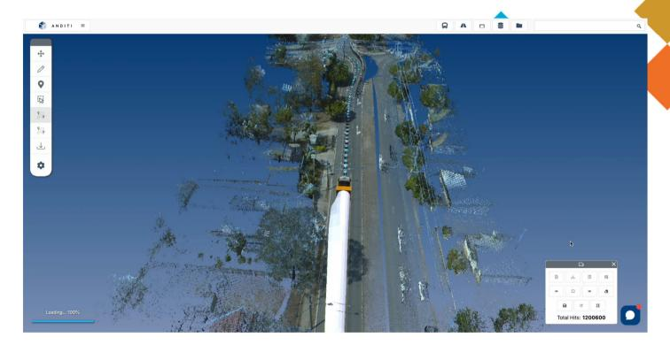
Ability to build vehicle model simply and drop into the point cloud- with dimensions, number of trailers, front/rear drive etc
