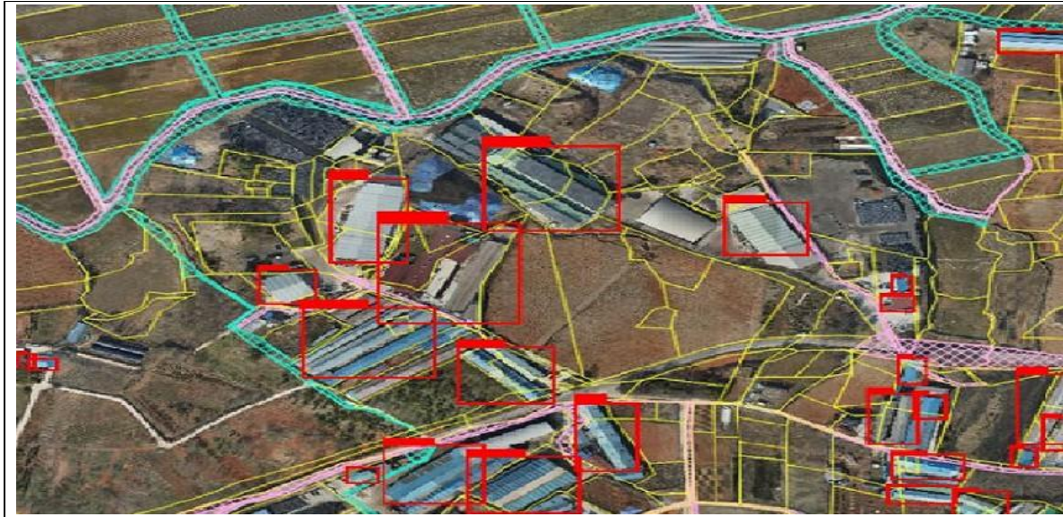
Figure 6. Object Detection of Roads, Waterways, and Building Conditions
