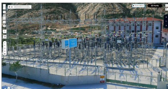
Figure 1: 3D Model of Substation Center
