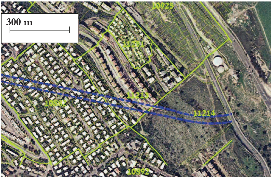
Figure 1: Orthophoto of a part of Haifa and the Carmel Tunnel layout (broken line), combined with blocks and parcels derived from the National GIS.
