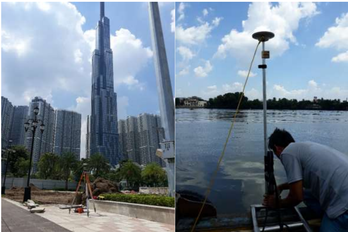
Figure 2. The base station on the point BM00 & AT502 Antenna on the vessel
