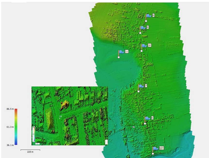
Figure 1.1.3 The Digital Terrain Model obtained from the cloud of points processing
