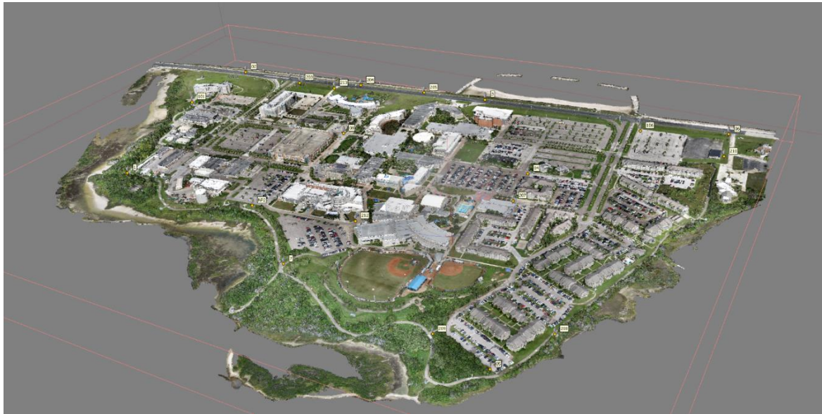
Figure 9: 3D point cloud of TAMUCC campus created from imagery taken using Wingtra.
