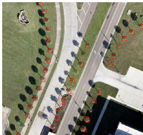
Figure 16: Palm tree detection in UAS imagery using a deep learning method.
