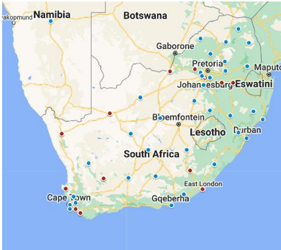
Figure 7 Map showing TRIGNET stations used to determine both the velocity and datum grids. Red dots were used as test points, while both the blue and red dots were used to constrain the grids.
