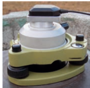
Fig. 10: Low-price u-blox ANN-MS antenna with adapter.
