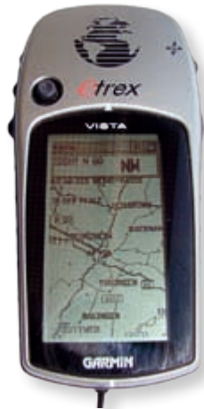
Fig. 7: Garmin eTrex Vista (raw phase data available, format not documented).
